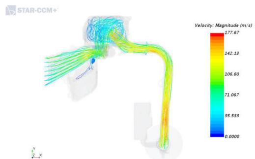
**Figure 4.3: Stream Line Passes Through Inside the Air Intake System**
